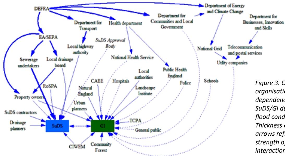
Figure 3. Cyber organisational dependencies for SuDS/GI during the flood condition. Thickness of the arrows reflect the strength of the interactions
