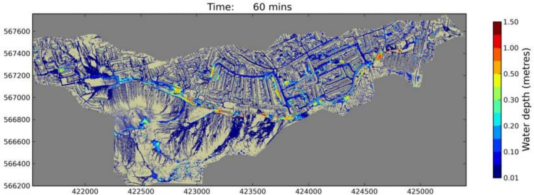
Figure 4-13. Result of simulation 17 (RP 100 y, duration 1 h, sewer network not active).
