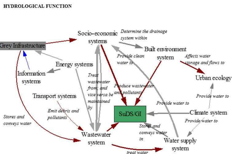
**Figure 1** Interdependencies of SuDS/GI onto other urban systems under the non-flood condition
