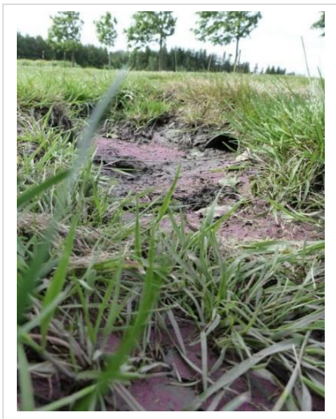
Tracer deposition within an urban established swale
