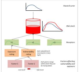
Figure 4: Model schematic showing how a 'risk curve' is derived from the combinations of the risk to each receptor at that location. The risk to each receptor is a function of its exposure and vulnerability, each of which can be changed by altering the relevant factors.
