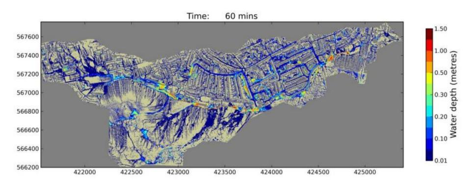
Figure 4-13. Result of simulation 17 (RP 100 y, duration 1 h, sewer network not active).
